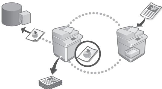
You can register a Windows server or the Advanced Space of another Canon multifunction printer as a connection destination. This enables you to use the machine to print data that is on the connection destination.
