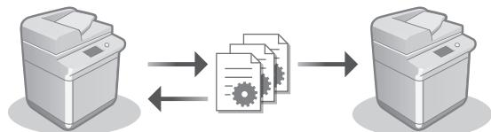
You can save (export) the settings data of another Canon multifunction printer to a computer. You can then import that settings data to the machine to skip the configuration procedure.
