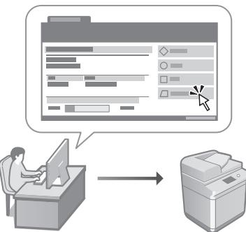
Remote UI allows this machine to be managed using the Web browser on a computer. You can use it to check the machine's operating status, change settings, and save items to the Address Book.
